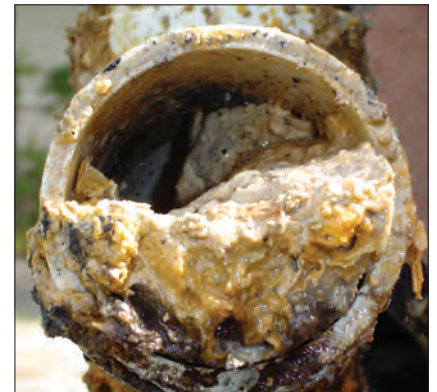
Fats, cooking oils, and grease can coat and clog pipes and cause sewer lines to back up into homes.
