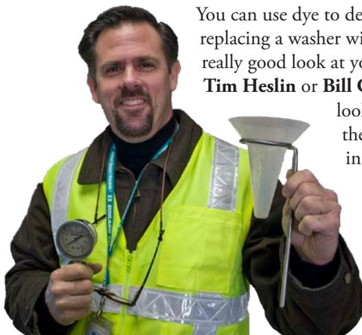
Tim Heslin holds up two of the devices he uses to test water pressure and irrigation coverage.
